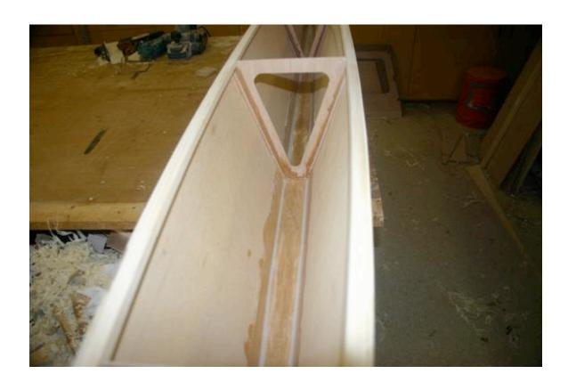
10) Test fit the notches for the sheer stringer with a scrap of 1/2" square wood, so the stringer will fit flush with top of the hull panel. Fit the stringers to the transom first, and then at bow. Apply thickened epoxy to the inside of the hull panels, and glue the stringers in place, using spring clamps to hold the stringer.
