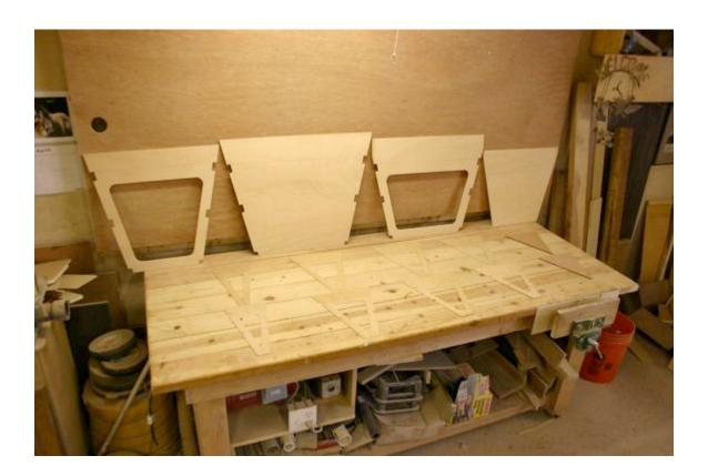
2) You will need a flat workbench 2' wide, by 16' long, which can be made from 2 x 4s and 1/2" plywood. Make sure it is straight, and not twisted. Any twist will be built into
