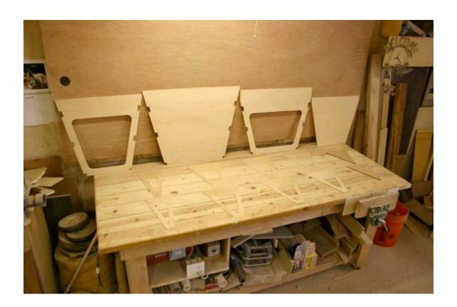
2) Draw a centerline on your workbench and measure the distance from the bow of the location of the frames. Draw a perpendicular line. Install the frames at each station with two screws. You can cut a small scrap of plywood to the 21-degree angle to hold the transom in place.
