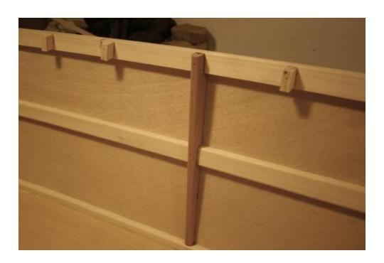
9) Fair out the deck structure so everything is flat. Scribe the fore and aft deck panels so they extend past the rounded pieces at the front and back of the cockpit. Glue in place and hold down the edges with masking tape. You can use some weights to hold them down in the middle until the glue dries. Fit pieces of 1/8" ply to cover the rest of the rail in the cockpit, and glue in place.
