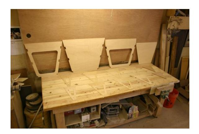
2) Draw a centerline on your workbench and measure the distance from the bow of the location of the frames. Draw a perpendicular line. Install the frames at each station with two screws. You can cut a small scrap of plywood to the 13-degree angle to hold the transom in place.
