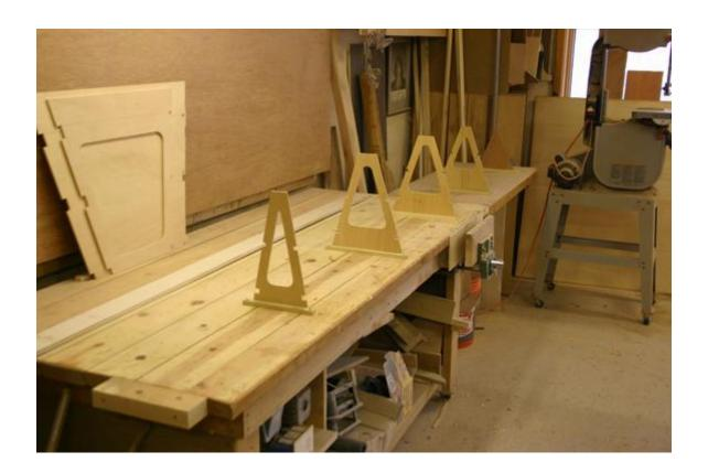
3) Scarf together the 1/8" plywood hull sides, so you have panels that are 13" wide by minimum of 10' 2" long. You will need 4 panels. Plans for a scarfing jig are included with the drawings.
