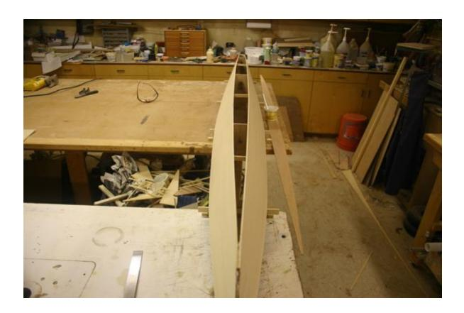
9) Unscrew the hull from the work bench, and turn it over. Using a fine-tooth saw, cut off the frames at deck level. Cut strips of 4 oz. fiberglass to fit in the bottom of the hull between the frames, wide enough to go up the sides at least 3/4". Put a radius of thickened epoxy in the corner where the sides meet the bottom. Put the strips of fiberglass in, and wet out with epoxy and a small brush.
