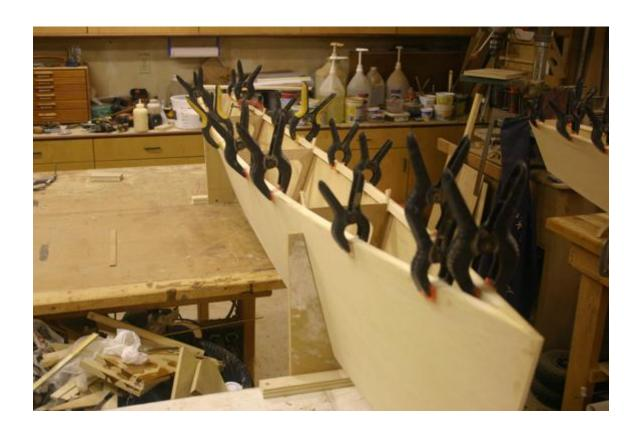
11) Fair out the sheer stringer and frames. Check the deck for flatness with a straight scrap of wood. Fit the two layers of 1/2" plywood for the beam attachment. The bottom layer fits under the sheer stringer, the top flush with the deck. Epoxy in place. Glue the  $1 \frac{1}{2}$ " x  $2 \frac{1}{2}$ " x  $2 \frac{1}{2}$ " block under the beam attachment.
