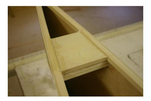
12) Scarf together two pieces of 1/8" plywood 11" wide by 10' 2" long for the decks. Make sure the deck structure of the amas is fair. Lay the plywood on the deck, scribe the panels, and cut out. Roll a coat of epoxy on the bottom of the deck plywood, and put thickened epoxy on the deck structure. Carefully lay the panel in place, and secure with masking tape.
